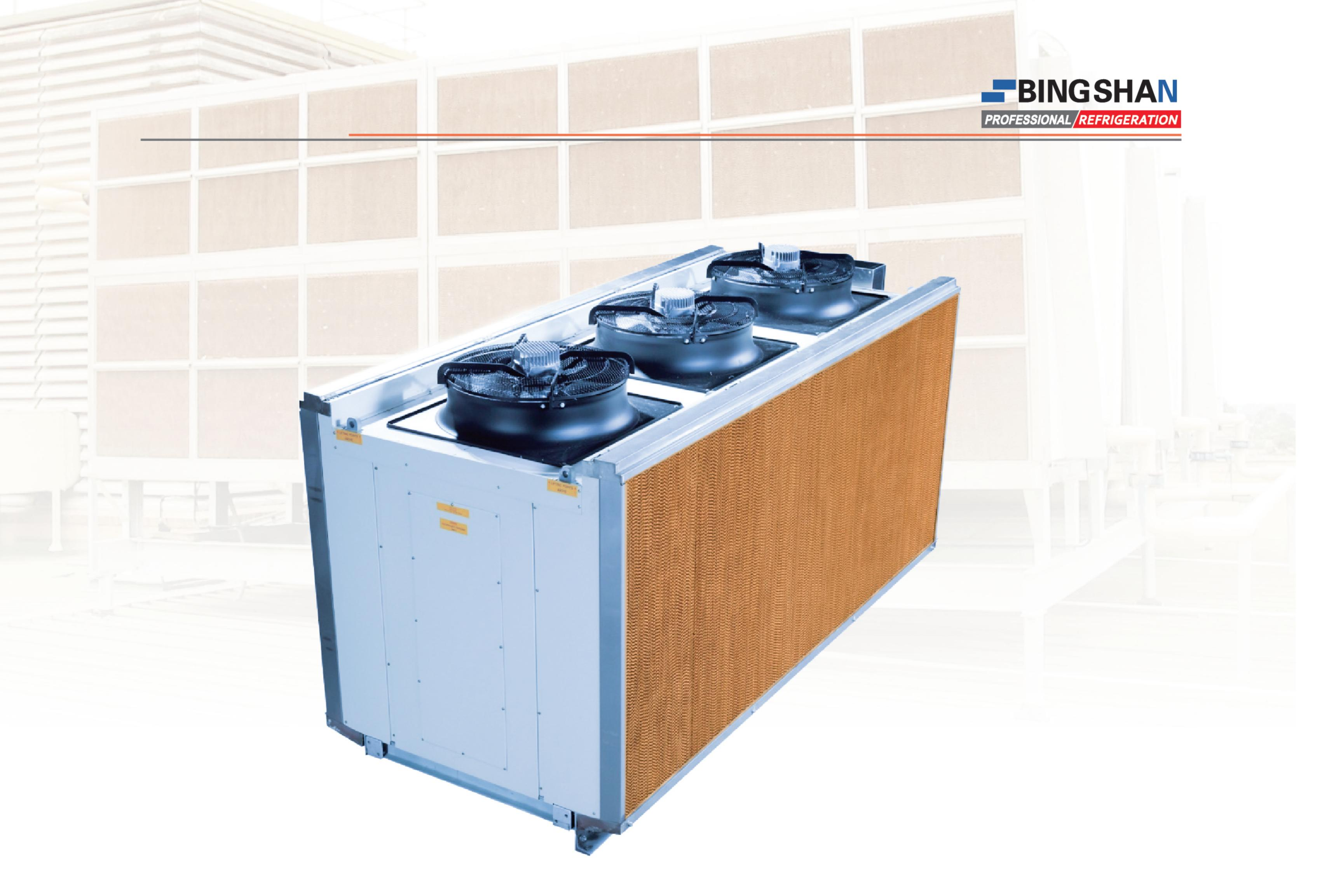
The Adiabatic cooler is a combination of a dry cooler and an adiabatic cooling track before the air inlet. Adiabatic pre-cooling is activated then the water outlet temperature is higher than needed. The cooling medium is cooled to below the ambient air temperature completely abacterial and without water treatment. The system works on the adiabatic principle of heat rejection. By extracting energy from the air
