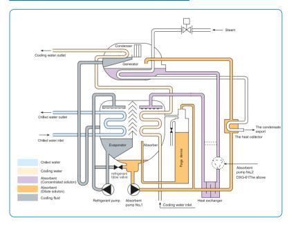
Our DXG Steam-fired Single Effect LiBr Absorption Chiller is made of evaporator, absorber, condenser, generator, heat exchanger, heat reclaimer, solution pump and refrigerant pump etc.
